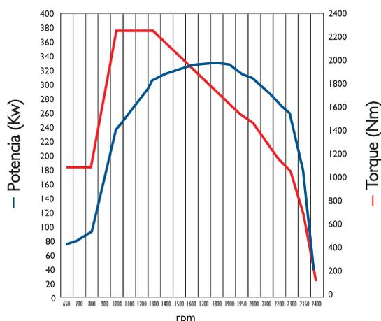
Potencia del motor: 324 kW (440 CV) @ 1 900 rpm
