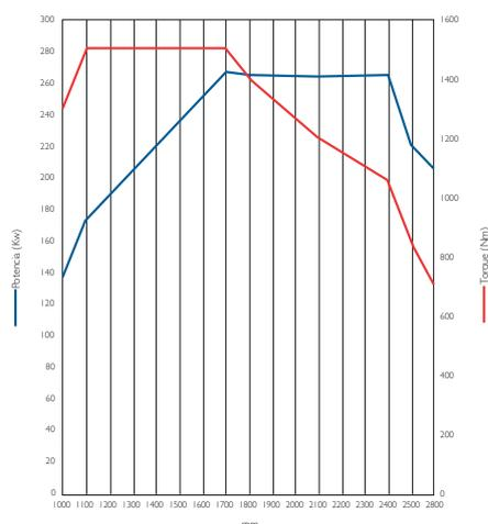
Potencia del motor: 265 kW (360 CV) @ 2 200 rpm
